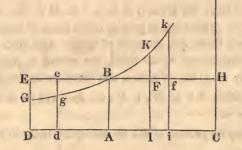
Describe the hyperbola G B K between the asymptotes A C and C H cutting the perpendiculars D E, d e, in G and g.
